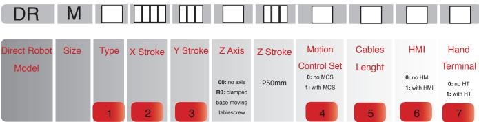
1 Choose the DIRECT ROBOT unit architecture g: gantry single y gv: gantry single y-z 2g: gantry double y 2gv: gantry double y-z sh: slide har
