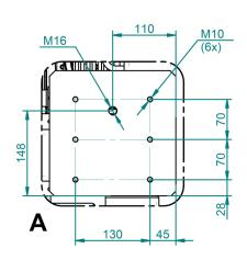
Dimensions can be modified according to application requirements
