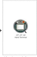
The motion control architecture is based on Core Pro environment; development environment has two main layers: PLC and Robotic. The hand terminal device allows to use at once robotic functions for fast and direct configuration of the motion part of the application. The PLC layer allows the configuration of the automation and interface part of the application.
